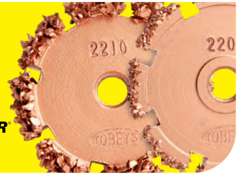
6082101 Contour cup rasp 50x25mm - 16 grit (A210/16)
