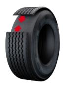
Retreading using conventional flat strips necessarily involves the presence of at least one splice. In addition to inevitably throwing the tyre off balance, this creates a weak point that can increase the likelihood of the tread detaching itself.
