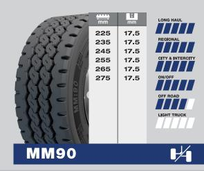
The MM90 is a dual-purpose tyre designed for both on and off-road use. It features a 4-rib design and open tapered grooves to reduce stone trapping.
