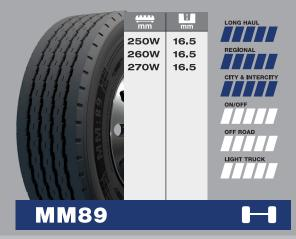
5 rib tread with broad tapered shoulders with added wing to withstand side scuffing on tandem wheel applications.
