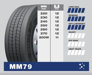
The MM79 is designed for trailers. It features the Milemaster compound, a light 5-running rib pattern that ensures even wear, cool running, and excellent mileage. Its wing technology assists in severe scuffing applications.
