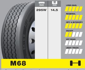
5-running rib pattern for even wear, cool running, mileage, and wing tech for severe scuffing
