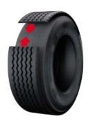
Retreading using conventional flat strips necessarily involves the presence of at least one splice. In addition to inevitably throwing the tyre off balance, this creates a weak point that can increase the likelihood of the thread detaching itself.
